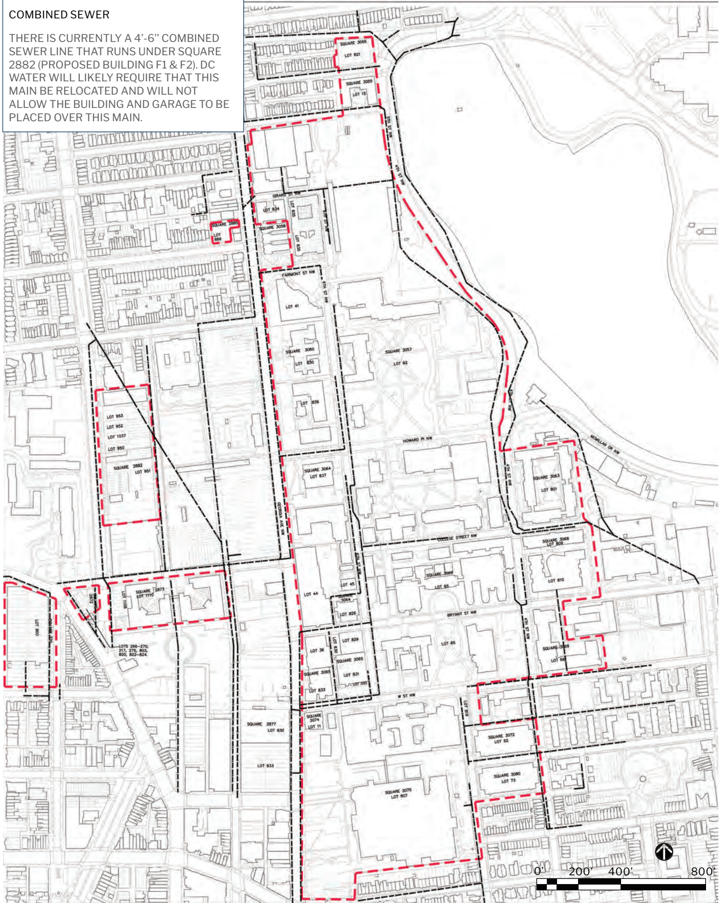
Figure 3.33: Existing Combined Sewer Distribution
